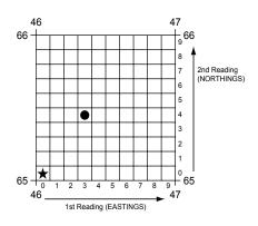
To give the six-figure grid reference, first identify the grid square, in this case 4665. The third figure is obtained by dividing the space between grid lines 46 and 47 into ten equal parts. Similarly, the sixth figure is obtained by a similar division of the gap between northings 65 and 66. This results in a grid reference of 463654 for the dot and 460650 for the star. It should be noted that the first tenth is 0 and the last tenth is 9 in the divided grid square.
